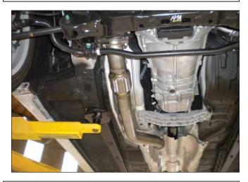
f. Front exhaust pipe installed.
