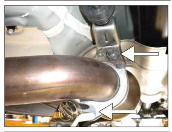
j. Remove the two nuts securing the OEM catalytic converter to the front exhaust pipe.
