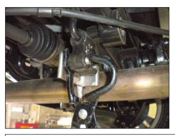
f. Unhook the hanger located on the rear exhaust pipe that was connected directly to the muffler by flipping the rubber isolator up.
