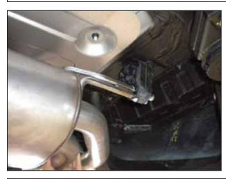
m. Install the driver side muffler hanger into the rubber isolator.
