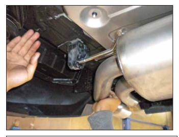
n. Install the passenger side muffler hanger into the rubber isolator.
