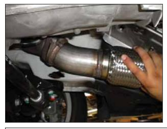
c. Align the front  $AEM^{\circledast}$  exhaust pipe with the studs located on the turbo manifold
