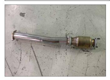
g. Create an assembly outside of the vehicle with the middle AEM<sup>®</sup> exhaust pipe and the OEM catalytic converter using the two supplied nuts (1-1005) and the OEM metal gasket between the two parts.
