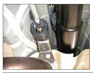
I. Unhook the hanger from the rubber isolator located on the rear flange of the front exhaust pipe.
