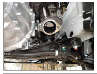
b. Install the OEM exhaust gasket on the turbo manifold.
