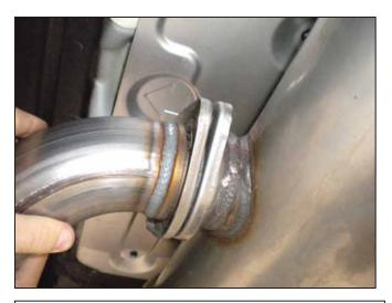
o. Align the muffler with the rear exhaust pipe.
