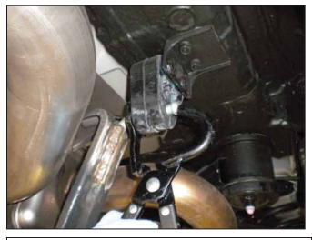
c. Unhook the passenger side hanger from the rubber isolator.
