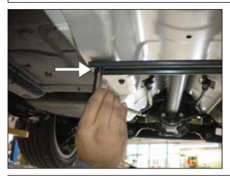
m. Remove the passenger side bolt securing the brace shown.
