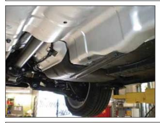
p. OEM exhaust system removed.
