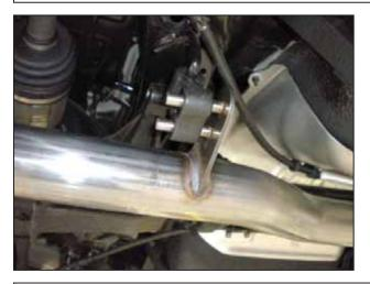
j. Install the rear AEM<sup>®</sup> exhaust pipe aligning the hanger with the rubber isolator.
