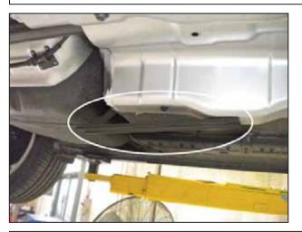
o. Rotate the brace out of the way.
