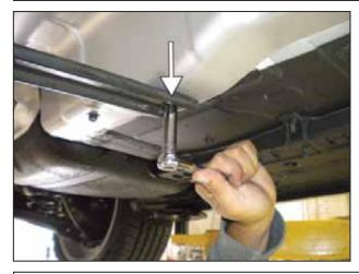
n. Loosen but do not remove the driver side bolt securing the brace.
