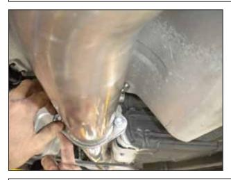
k. Install the two supplied M10 nuts (RHNA-M10X125) on the bolts installed in step 3i.
