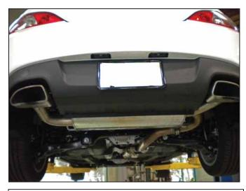
a. Stock exhaust system installed.
