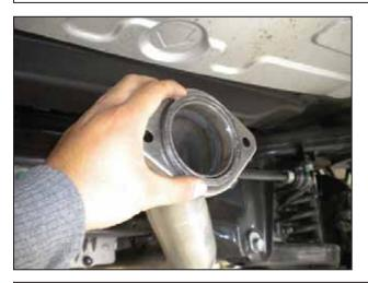
I. Install the supplied gasket (RM-CB81) on the end of the rear exhaust pipe.
