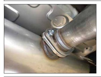
p. Secure the rear exhaust pipe to the muffler using the supplied M10X1.25X25 bolts (RHBA-M10X125X25) and nuts (RHNA-M10X125).
