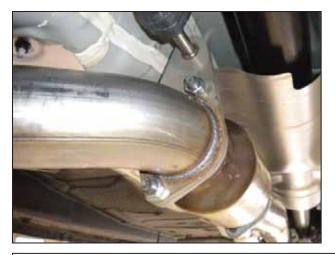
h. Connect the OEM catalytic converter/AEM<sup>®</sup> middle exhaust pipe assembly to the front AEM<sup>®</sup> exhaust pipe. Sandwich the OEM metal exhaust gasket between the two pipes and secure using the two supplied nuts (1-1005).
