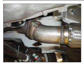
e. Install the two supplied nuts (1-1005) on the studs as shown, keep loose.
