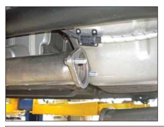
i. Install the supplied M10X1.25X35mm bolts (RHBA-M10X125X35) and the supplied gasket (RM-CB83) as shown.
