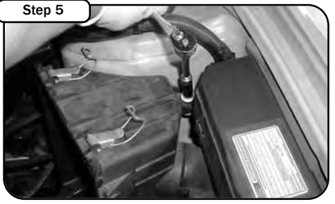
Step 5 Remove the 10mm bolt that supports the other half of the airbox and remove the rest of the airbox.
