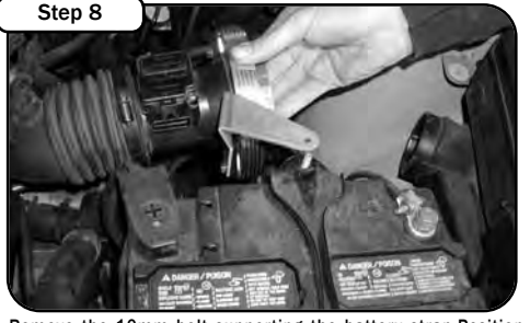
Step 8 Remove the 10mm bolt supporting the battery strap. Position the intake assembly into the engine bay. Line up the hole on the bracket with the battery bracket as shown, reinstall bolt and tighten bolt to secure assembly.
