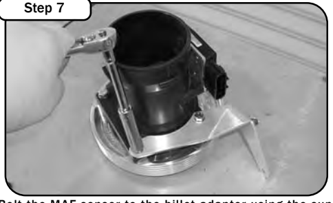
Step 7 Bolt the MAF sensor to the billet adaptor using the supplied M6 screws and washers. On the right side of the sensor place the aluminum bracket and fasten to assembly as shown in photo.
