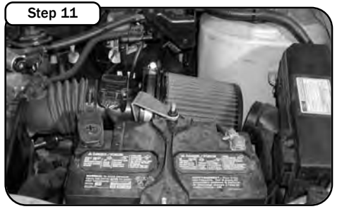
Step 11 Make sure all clamps are tight and that all electrical components are secure. Re-check and after a few hours of operation. Place the included CARB EO Sticker on or near the intake system on a smooth, clean surface. E.O. identification label is required in passing the Smog Check Inspection.
