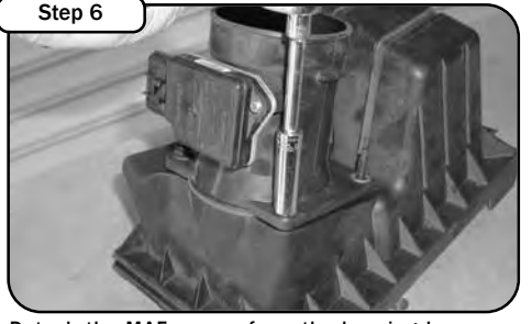
Step 6 Detach the MAF sensor from the housing by removing the four 10mm screws.
