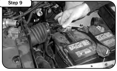
Step 9 Reconnect the Maf sensor and tighten down the hose clamp on the intake pipe
