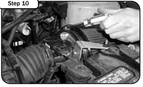
Step 10 Install the pre-oiled filter in the housing and tighten down clamp. DO-NOT use any oil or grease.
