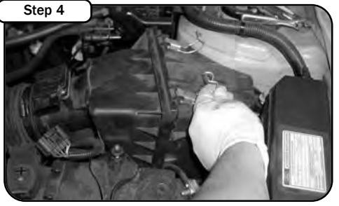
Step 4 Unclip the two mounting clips located on the side of the airbox. Lift the top half of the airbox out and remove..
