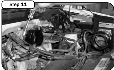
Install the hump hose and clamps on the air filter housing and install the 3" straight coupler and clamp on the throttle body
