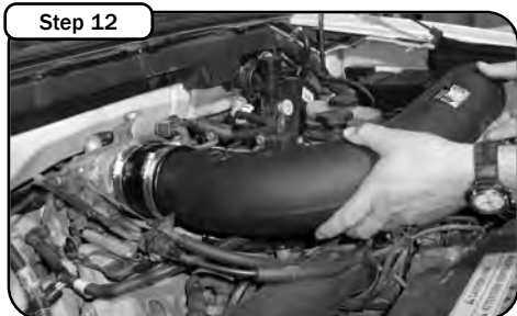
Install the smaller end of the intake tube into the throttle body coupler and insert other end into the hump coupler on the hosing. Tighten down clamps on both couplers.
