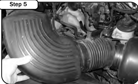
Unplug the IAT sensor and remove the intake duct from the engine. On some 04-05 models the IAT sensor is not present.
