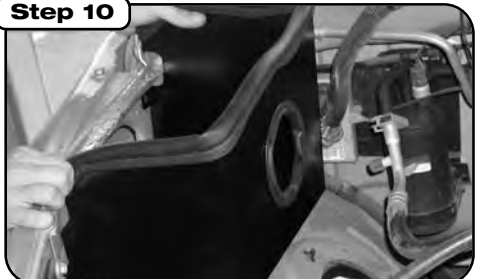
Install large housing trim seal to top of housing and small trim seal to tube inlet. Attach filter housing to inner fender-well with the three specified bolts.
