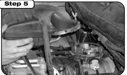
Once clamp is loose, pull up and out. Reuse existing gasket.
