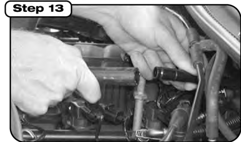
Connect supplied vent hose to nipple at intake tube and at breather vent tube. Note: no clamps are required.
