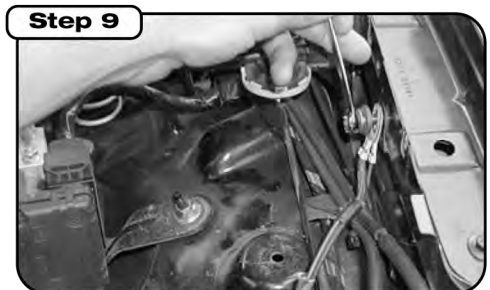
Remove ground strap at inner driver-side fender well. (Keep bolt for installing filter housing.)
