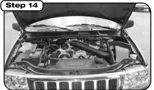
Place enclosed CARB EO sticker on a clean/smooth surface on or near the intake system. EO identification label is required in passing Smog Check inspection. Make sure all hoses and clamps are tight and that all electrical components are secure. Re-check after a few hours of operation.
