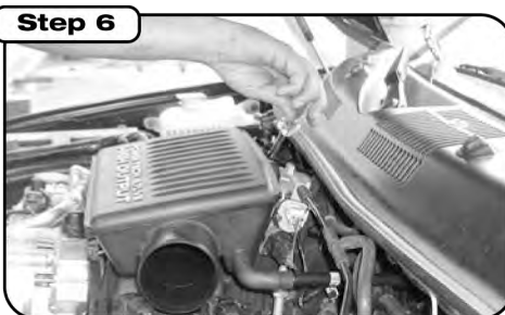
Loosen clamp at throttle body and remove resonator box.
