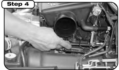
Unbolt resonator at manifold (Two bolts, opposite sides).
