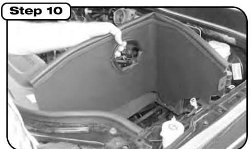
Before installing housing, apply large trim seal to top of housing and small trim seal to tube inlet. Install filter housing using supplied hardware on lower mounts.
