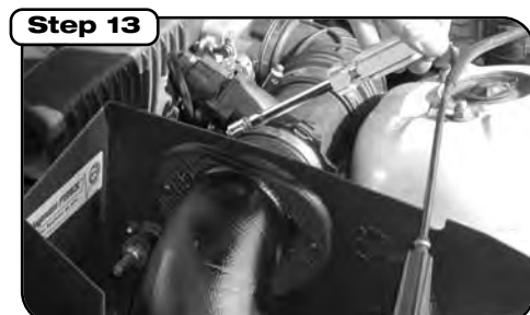
Tighten clamp on tube and align bolt holes on tube to shield.
