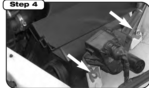
Remove two nuts that hold the cruise control module to the airbox with 10mm socket or wrench located on back side of airbox..
