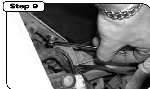
Use provided M6 screw and washer to tighten shield to front core support.
