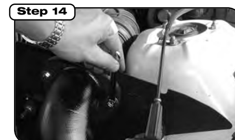
Use the three longest M6 bolts and washers provided to bolt the tube flange to the shield.
