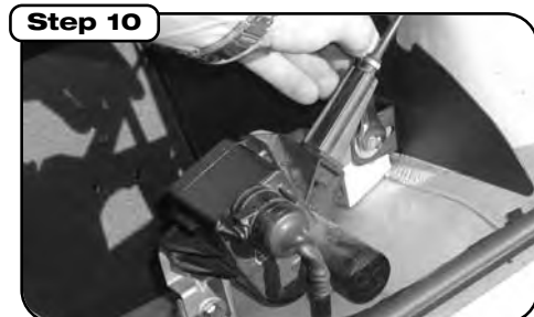
Place cruise control module back in location and use M6 bolts, screws, washers and lock washers supplied with kit.
