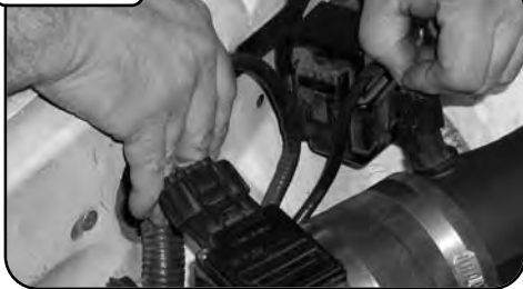
Connect wire harnesses to MAF sensor and temp sensor.
