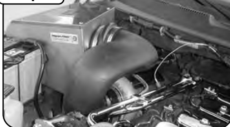
Make sure all clamps are tight and that all electrical components are secure. Check and retighten connections and filter after a few hours of operation.
