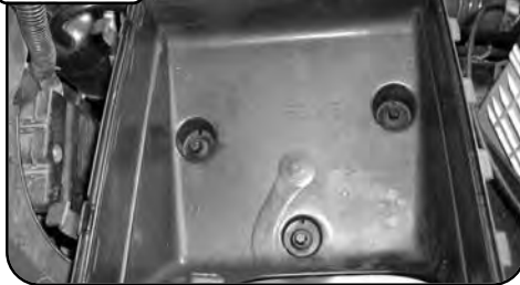
Remove lower half of filter box, unscrew 3 inserts and transfer inserts to new filter housing.
