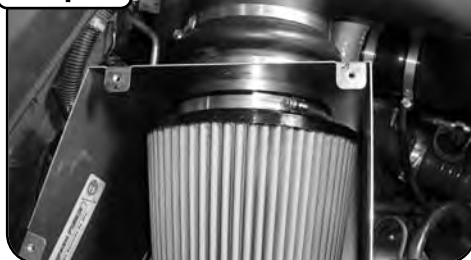
Install factory pre-oiled filter into housing. Install cover and make a final check for loose clamps, pinched wires etc. before starting engine.
