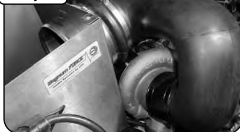
Slip boots over intake tube and install on turbo and filter housing. It may be easier to install clamps after tube is in position. If filter restriction gauge is desired, drill an 11/16 hole with a woodworking spade bit and transfer grommet and sensor to new intake tube. Sensor should be placed near larger end of tube for accurate results.
