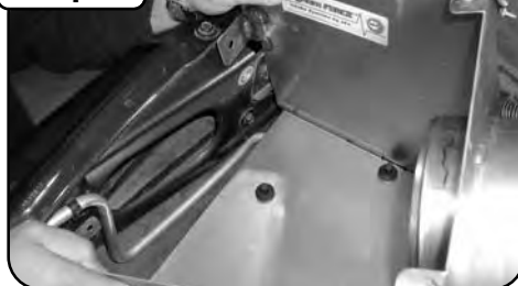
Lower housing into place, tab for ground screw tucks behind A/C line first, then lower to clear turbo housing. Housing should clear A/C line, line up rubber mounts and secure by pushing down hard or screwing mounts in. Install fender brace screw and ground screw and wire.
