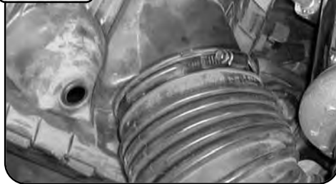
Loosen clamp at turbo inlet and remove top half of filter box and filter element.
