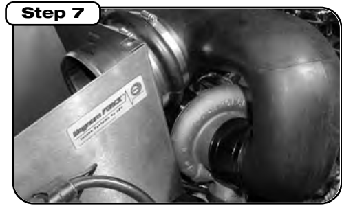
Step 7 Slip boots over intake tube and install on turbo and filter housing. It may be easier to install clamps after tube is in position. If filter restriction gauge is desired, drill an 11/16 hole with a woodworking spade bit and transfer grommet and sensor to new intake tube. Sensor should be placed near larger end of tube for accurate results.
