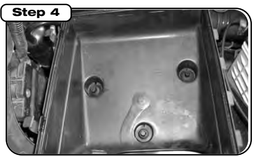
Step 4 Remove lower half of filter box, unscrew 3 inserts and transfer inserts to new filter housing.
