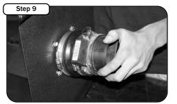
Slide the MAF sensor, clamps (#072 and #064), and reducer coupler (05-00020) on the air filter adaptor. Do not tighten the clamps at this time.
