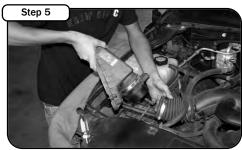
Loosen the hose clamp connecting the MAF sensor to the airbox. Remove upper portion of the airbox and MAF Sensor. Carefully set MAF sensor to the side for later use.
