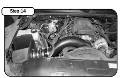
Place enclosed CARB EO sticker on a clean/smooth surface on or near the intake system. EO identification label is required in passing the Smog Check inspection. Make sure all hoses and clamps are tight and that all electrical components are secure. Reconnect the battery at ths time.
