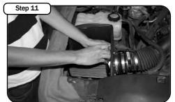
Install intake filter into housing. Re-connect the MAF sensor. Your Stage 1 installation is now complete. Make sure you tighten all clamps and check all electrical connections. Re-check periodically. Continue onto steps 11-13 to install Stage 2.
