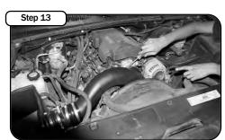
Place straight coupler (05-00421) with clamps (#60) on throttle body and the hump coupler (05-00565) with clamps (#064) on the MAF sensor. Install intake tube. Tighten and secure all hose clamps. Rotate fan to make sure there is sufficient clearance between the intake tube and the fan.
