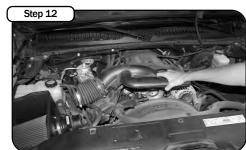
Remove the factory intake tube out of the engine bay. On some models there is a plastic tab you have to disconnect that secures the tube to the wiring harness.
