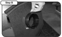
Place the air filter adaptor inside the housing. Secure the adaptor with the M6 button head screws and M6 wavy washers provided.
