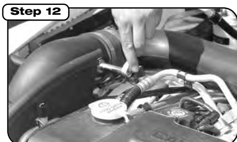
With intake tube in place mount tube to housing using supplied rubber/metal washer on each side of housing tab and split lock washer at bolt head. DO NOT OVER TIGHTEN.
