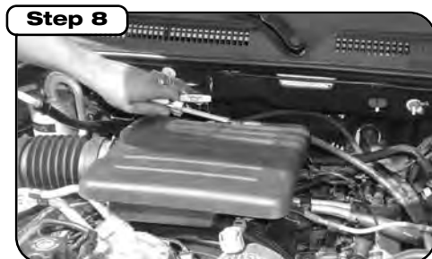
Loosen hose clamp at throttle body and pull up and out.
