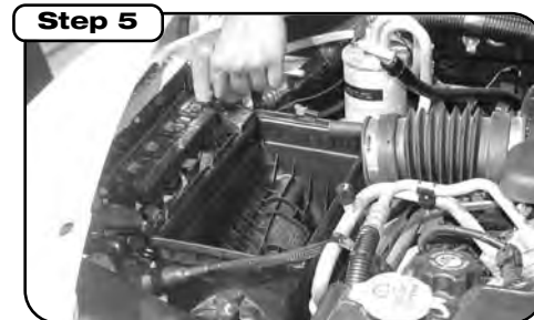
Loosen and remove bolt (one only) from OE filter box.
