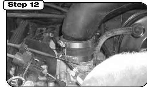
Install intake tube onto throttle body making sure tube is completely resting on throttle body to ensure proper hood clearance. Tighten clamps to secure tube.
