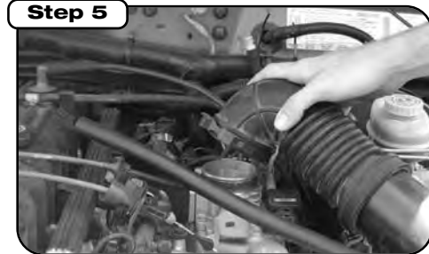
Loosen clamp at throttle body and remove.
