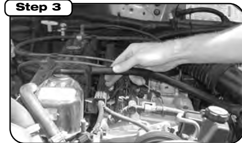
Remove breather tube from valve cover vent.
