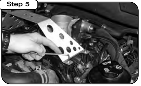
Install the intake tube support bracket to the intake manifold and fasten with the supplied M6 button head screws and washers.
