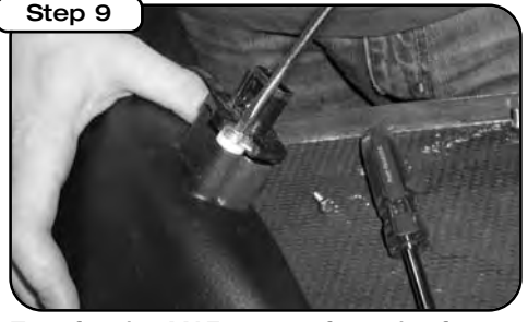
Transfer the MAF sensor from the factory airbox to the new intake tube. Make sure you use the provided spacer and gasket.
