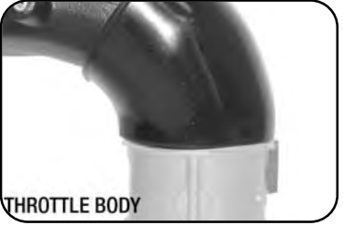
Position coupler and clamps over throttle body (3.5" x 4.0") (clamps removed for clarification). The smaller (3.5") end of the coupler goes over the throttle body. The (4") end of the coupler goes around the intake tube.
