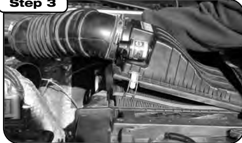
Loosen clamp from stock intake tube (at engine side), disconnect plug to filter minder and undo clips to remove top of OE air box.
