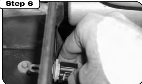
Twist and remove temperature sensor from air box. Being careful not to damage sensor.
