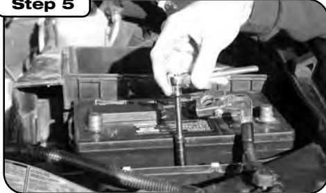
Remove battery hold down clamp from OE battery tray.
