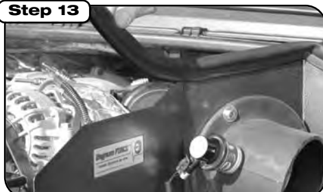
Install trim seal on housing.
