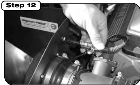
Install temperature sensor.
