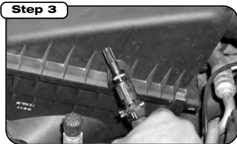
Remove temperature sensor from stock air box
