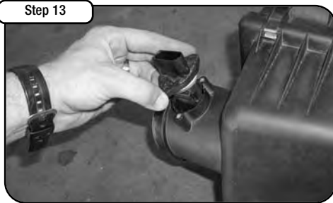
Using provided Torx bit, remove MAF sensor from factory airbox and re-install into aluminum adapter using (2) provided M4 screws. Re-connect factory harness to MAF sensor.
