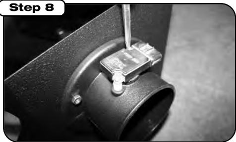
Insert mass air flow sensor back into housing and tighten down using 2 screws, 2 nylon spacers and gasket provided between sensor and tube.
