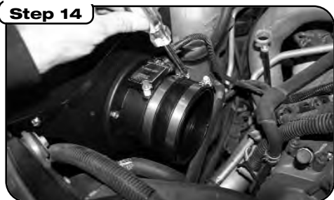
Install provided couplers. Be sure to install the small end of the tapered coupler to the turbo inlet housing. The remaining coupler must be installed with the smaller inner diameter attached to the heat shield, and the larger inner diameter will receive the Stage II tube. Install Stage II tube into couplers. Reposition duct clamps if additional clearance is necessary.
