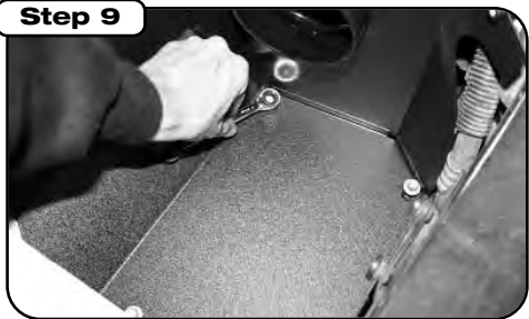
Install housing and re-use 4 bolts from step 6. Fasten securely.
