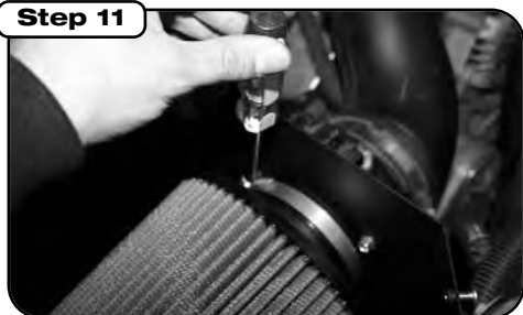
Install filter and tighten clamp. Do not use oil or grease.
