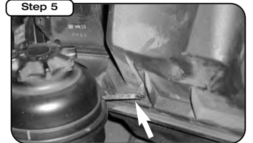
Detach resonator box from stock air box assembly using 8mm socket.
