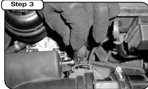
Unclip MAS (Mass Air Sensor) from air box using flathead screwdriver.
