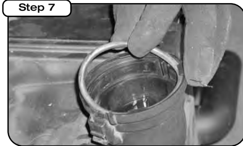
Carefully remove o-ring from stock air box.
