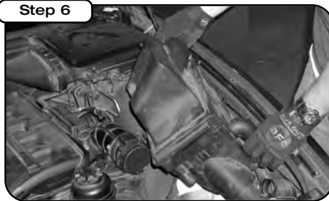
Remove OE air box from vehicle.
