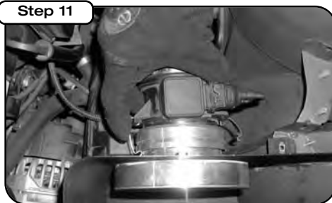
Attach spring clips that are supplied in kit to MAS and clip onto billet adapter.
