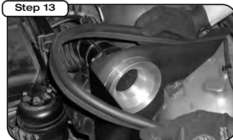
Install trim seal.
