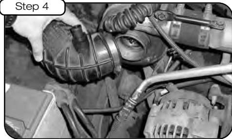
Remove factory rubber elbow at turbo.
