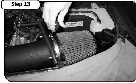
Install and tighten your pre-oiled filter. Do not use any grease or oil.
