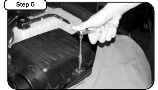
Remove the 10mm screw securing the airbox to the vehicle. Save for re-use later.
