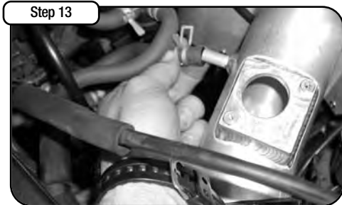
Connect remaining VSV vacuum line to the nipple in the intake tube.
