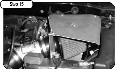
Place enclosed CARB EO sticker on a clean/smooth surface on or near the intake system. EO identification label is required in passing the Smog Check inspection. Your installation is now complete. Tighten all connections and clamps. Re-check after a few hours.
