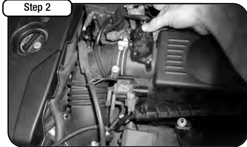
Disconnect wiring harnesses leading to Mass Airflow Sensor, VSV valves located to either side of MAS on factory airbox (indicated by arrows). On the brown harness toward the front end of the car, place provided rubber cap over harness lead.
