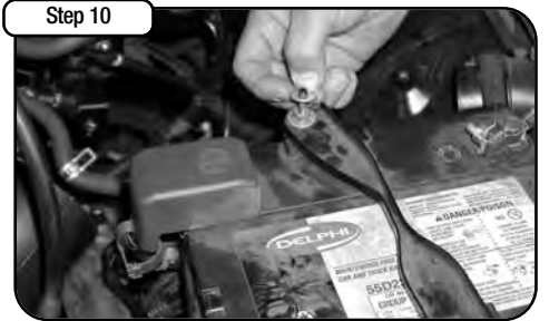
Place wave washer on TOP of battery hold-down nut.
