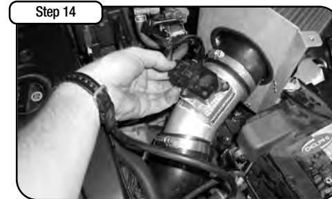
Remove the MAS from the factory airbox and re-install on aFe intake tube using provided hardware. Reconnect factory wiring harness to the MAS.
