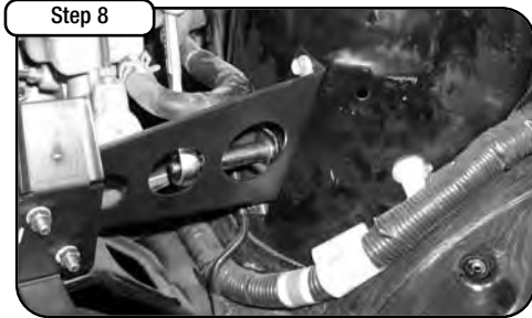
Bracket is to be installed in shock tower using the existing indicated bolts. NOTE: On cars equipped with cruise control, lower bracket should be sandwiched between cruise control bracket and shock tower. Upper bracket will use grounding bolt hole, but ground strap will be left off and re-attached later.
