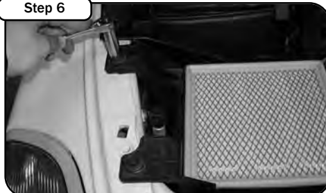
Step 6 Remove 2 screws on side fender well area and remove lower portion of airbox.
