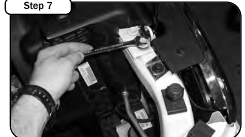
Step 7 Remove 13mm screw from radiator core support. This will be reused once heat shield is installed.
