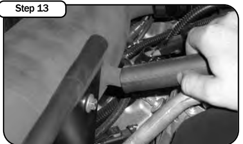
Step 13 Once tube is set into place fasten securely using supplied M6 x 1 x 16 screw and cushioned washer. Attach new vent line to tube and to oil fill chamber (On 4.7L engine you must trim hose to 13" for proper fit).
