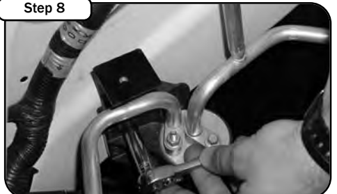
Step 8 Loosen screw but do not remove completely. Slide bracket that was supplied in the kit into place and retighten screw. This new bracket is placed in between the accumulator bracket and side fender well.
