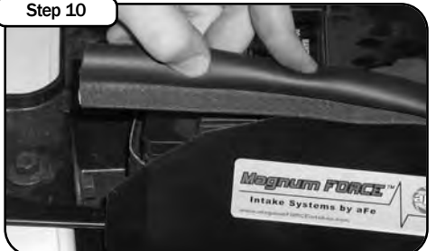
Step 10 Install trim seal onto intake housing.
