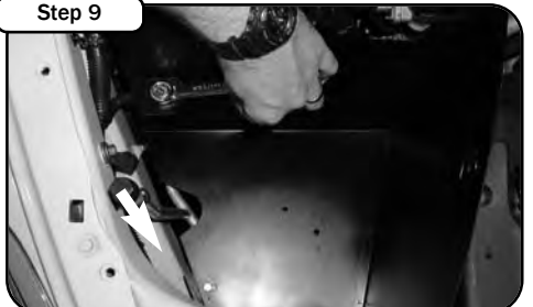
Step 9 Place intake housing into vehicle and fasten down securely reusing core support screw from step 7 and use M6 x 1 x 12 for the bottom screw.
