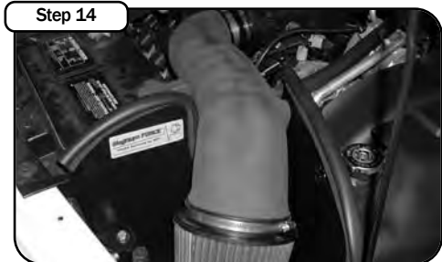
Step 14 Place enclosed CARB EO sticker on a clean/smooth surface on or near the intake system. EO identification label is required in passing the Smog Check inspection. Your installation is now complete. Tighten all connections and clamps. Re-check after a few hours.
