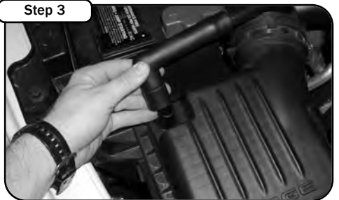
Step 3 Remove crank case breather line from airbox and oil fill chamber.
