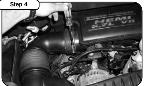
Step 4 Loosen clamp where intake tube meets resonator box.
