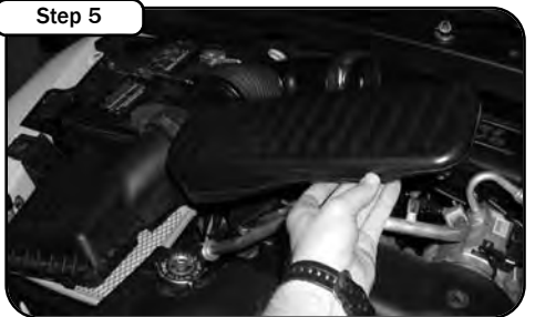
Step 5 Undo clips that hold stock intake box lid on and remove this complete assembly along with stock intake tube.
