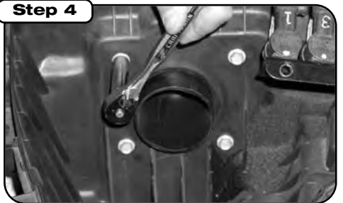
Loosen and remove 4 screws that hold stock intake tube to airbox.
