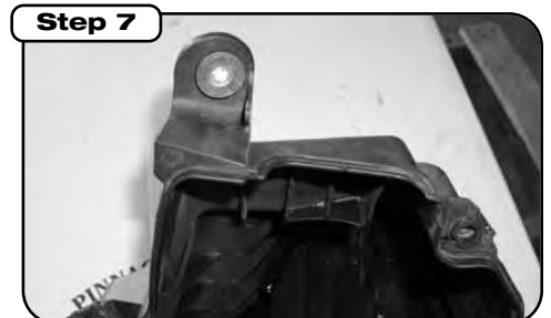
From the stock airbox, remove 1 washer and 1 rubber grommet and insert into new housing provided taking note of orientation of the washer.
