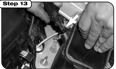
Remove air temperature sensor from stock intake housing that is sitting on the inner fenderwall area. This airbox piece will not be needed for kit.
