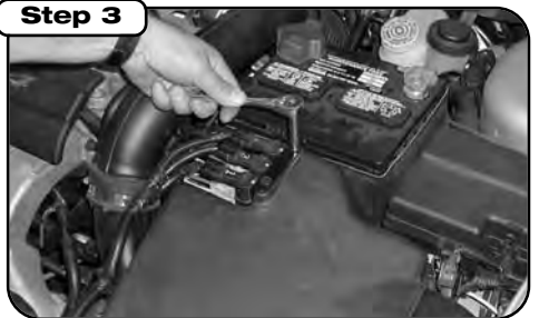
Loosen and remove solenoid mount, also loosen and remove stock intake lid.
