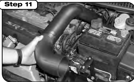
Install coupler onto the turbo side of intake tube, install tube into the vehicle and slide coupler onto turbo flange until coupler bottoms out on the lip of turbo inlet.
