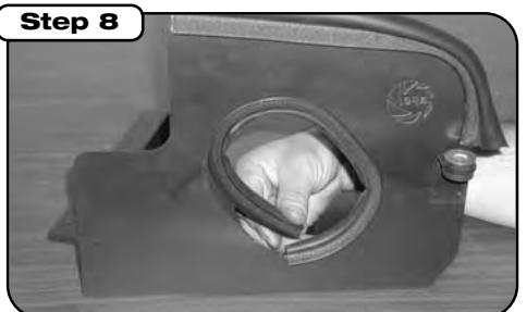
Before installing housing, install trim seal using 15" rubber grommet and insert into new housing provided taking note of orientation of the washer.
