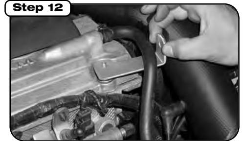
Remove plastic engine cover. Engine cover is held on by 2 grommets. Pull up cover evenly from both sides, making sure not to pull dramatically from one side so that engine cover will break. Using the aluminum bracket provided, place M6 washer onto stud, place bracket into place and secure tight with washer and nut provided. Align and install M6 bolt and lock washer to fasten bracket to the tube.
