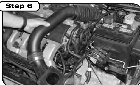
Loosen clamp on turbo inlet side of tube and remove stock intake tube from vehicle. Disconnect vent hoses from intake tube. Save as these will be reused.
