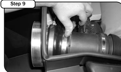
Slide the urethane coupler and hose clamps over the billet adaptor and reinstall the MAF sensor, tighten down all the clamps.
