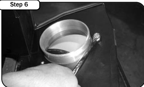
Assemble the new air filter housing by mounting the billet air filter adaptor to the housing and securing the adaptor with the 5 button head screws.
