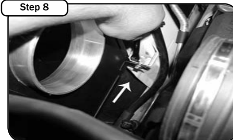
Line up the mounting tab to the airbox support brackets. Install the M6 bolt and washers and tighten down.
