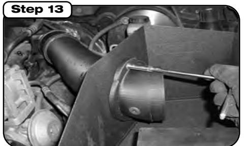
Using provided hardware, secure tube flange to heat shield. After tube has been secured to heat shield, tighten clamp holding the coupler to the tube.
