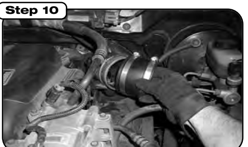
Place provided clamps loosely over provided coupler and place onto factory turbo inlet elbow
