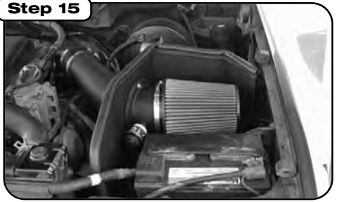
Place enclosed CARB EO sticker on a clean/smooth surface on or near the intake system. EO identification label is required in passing the Smog Check Inspection. Complete kit installed.
