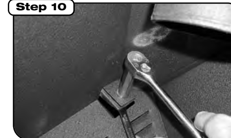
Using provided bolts, locking nuts and washers on both sides of the bolt, fasten lower tab on heat shield and slotted hole to the existing rubber mounts. Be careful not to over-tighten, it is only necessary that the rubber mounts be slightly compressed. Fully tighten shroud.
