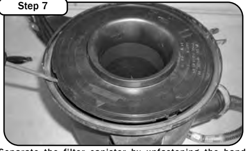
Step 7 Separate the filter canister by unfastening the band clamp and removing the air filter, disconnect the harness from the MAF sensor. Unbolt the MAF Sensor from the filter base and the short wire harness set aside for later use
