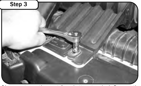
Step 3 Disconnect negative post from battery terminal. Remove the (4) 8mm bolts that hold the factory air intake assembly (set these bolts to the side you will be reusing these later).
