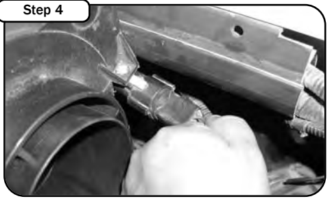
Step 4 Loosen the factory hose clamp with a nut driver or screwdriver connecting the black rubber intake pipe to the factory air filter housing. Unplug MAF sensor from harness and remove connector from the bracket located on side of air box by pulling straight out.
