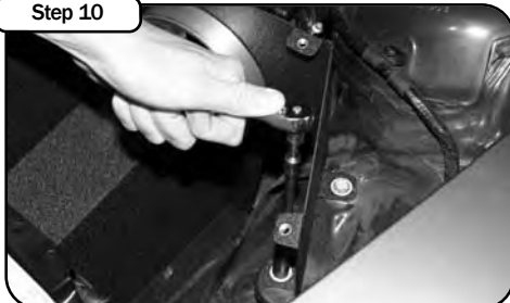
Re-install the two screws removed in step 4. Tighten down assembly.
