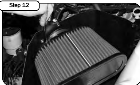
Step 12 Install and tighten your pre-oiled filter. Do not use any grease or oil.
