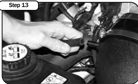
Step 13 Connect rubber breather hose to the factory vent location on the side of the valve cover and connect the other end to the side of the intake tube. Do not use any grease or oil.
