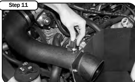
Step 11 Re-connect the MAF sensor to the wiring harness. make sure the red clip is pushed down to secure the harness.
