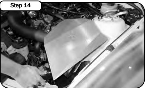
Step 14 Place the housing lid over the airbox and fasten with the supplied button head screws. Verify filter clearance with cover.
