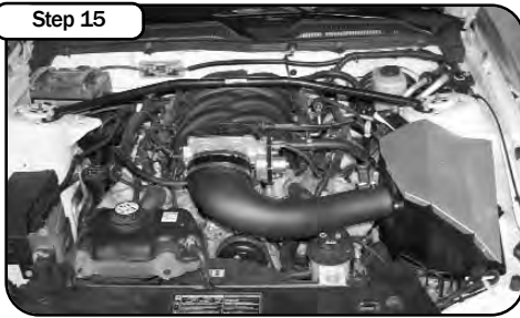
Step 15 Place enclosed CARB EO sticker on a clean/smooth surface on or near the intake system. EO identification label is required in passing the Smog Check inspection. Your installation is now complete. Tighten all connections and clamps. Re-check after a few hours.
