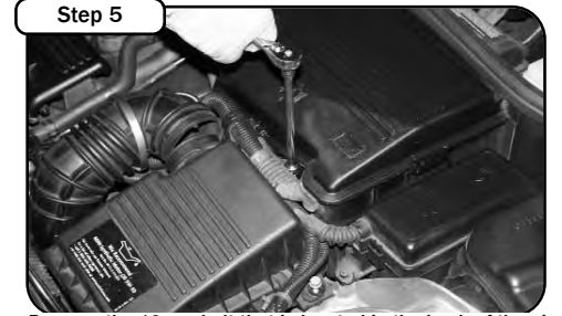
Remove the 10mm bolt that is located in the back of the air box securing the battery tray in place. Set the bolt to the side for later use.
