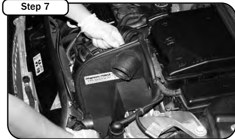
Position the new housing into the engine bay. Place the trim seal along the edge of the housing.
