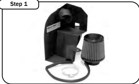
Complete intake system.
