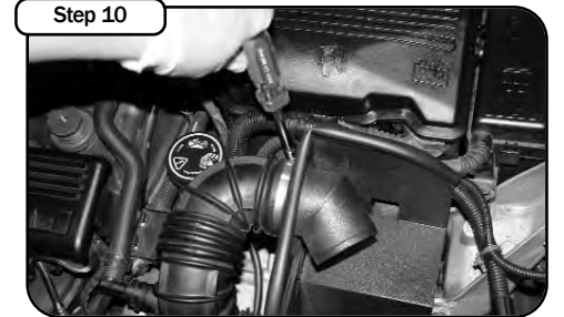
Place the new #044 clamp on the intake duct and tighten assembly to the housing inlet.
