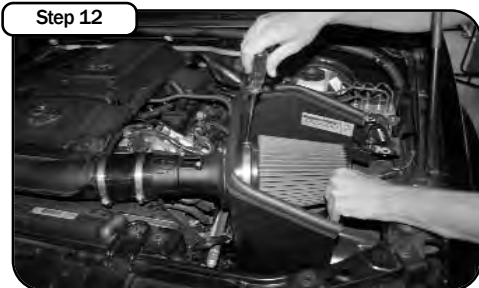
Step 12 Install the pre oiled air filter. Do not use any grease or oil. Secure with the provided clamp.
