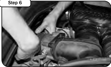
Step 6 Install the smaller 3" coupler and clamps on the throttle body. Do not tighten clamps at this time.
