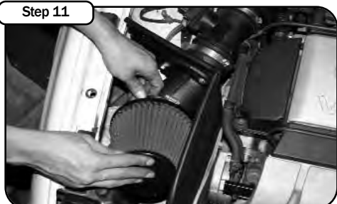
Step 11 Install the new air filter into the housing secure the filter with the provided clamp. The air filter is pre oiled from the factory.
