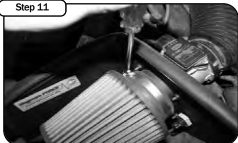
Step 11 Install filter and tighten clamp using a 5/16 nut driver. Reconnect factory intake hose to MAF sensor. Reconnect MAF sensor and temp sensor harness
