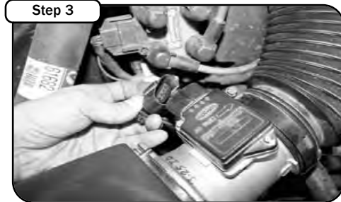
Step 3 Disconnect MAF sensor. Using 5/16 nut driver, loosen intake hose and disconnect.
