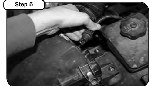
Step 5 Remove the factory air temp sensor. Set aside for re-installation.
