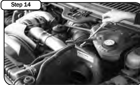
Step 14 Tighten both ends of the factory accordion coupler.
