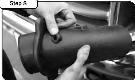
Step 8 Install Factory filter minder grommet into tube.
