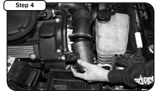
Remove both mass air sensors from the factory tubes using slotted screwdriver. Set aside for later use. Be sure to install sensors back to original side they were removed from.
