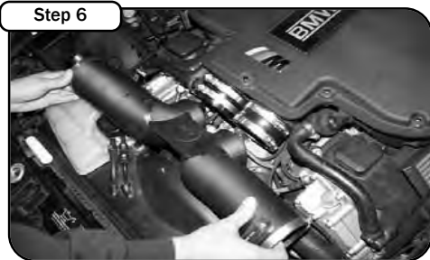
Using the 2 straight couplers provided in the kit install the high flow aFe intake tube.
