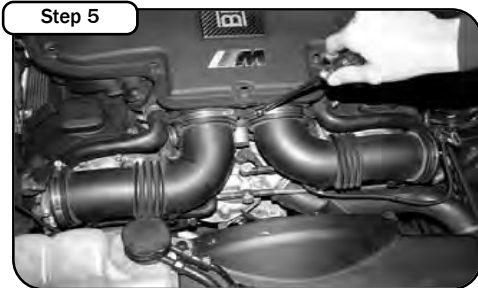
Remove both factory intake tubes from throttle body using a slotted screwdriver.
