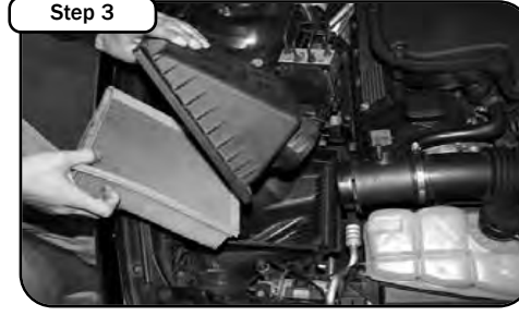
Remove clips from the mass air sensor and the air boxes and remove top half of air boxes and filters.
