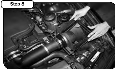
Install both air boxes using reducer couplers. Attach factory clips to secure to the air box and tighten clamps at coupler.
