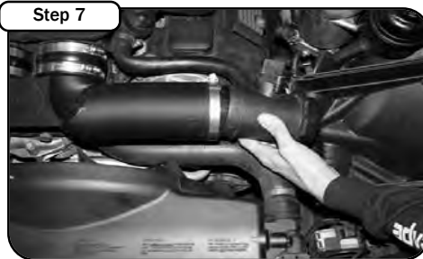
Install mass air sensors into the tube by pressing the sensor onto the tube. Tighten down provided #52 clamps.
