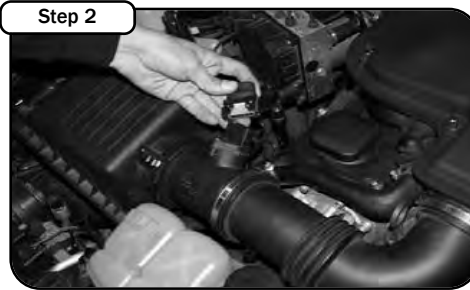
Unplug both Mass air sensor plugs from sensors.
