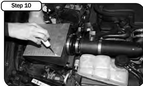
Using provided button head screws install covers with the aFe logo facing the front of the vehicle.
