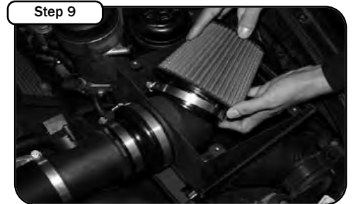
Install 2 provided High Flow aFe filters and tighten clamps.
