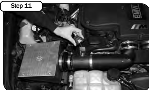
Re-connect both mass air sensor plugs.
