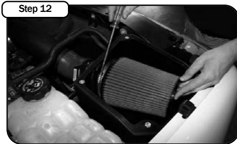
Step 12 Install filter into housing. Reconnect the MAS.
