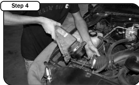
Step 4 Loosen the hose clamp connecting the MAF sensor to the air box. Remove upper portion of the air box and MAF sensor. Carefully set to the side for later use.
