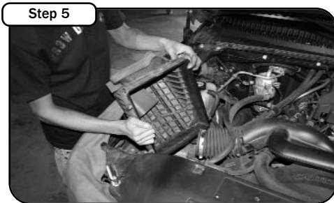
Step 5 Grab the lower portion of the air box. lift up and out. The box is secured with rubber gromets.
