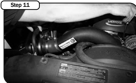
Step 11 Place straight coupler on throttle body (4"Dia x 2"Long) and elbow coupler on tube. Slide tube onto throttle body coupler. Attach elbow to MAS. Tighten clamps. Rotate fan to ensure sufficient clearance.
