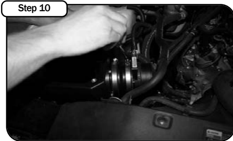
Step 10 Install MAS using supplied clamps and reducer coupler. Do not tighten clamps at this time.
