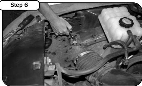
Step 6 Remove the four 10mm bolts that secure the air box base to the chassis. Save bolts for later use. Remove air box tray out of vehicle.
