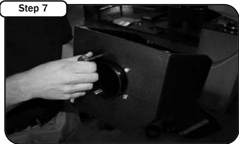
Step 7 Place the air filter adapter inside the housing. Secure the adapter with the supplied screws and washers.
