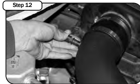
Step 12 Insert the air temp. sensor into the aFe intake tube. Re-connect the air temp. sensor plug.
