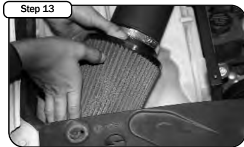
Step 13 Install the new aFe air filter onto the intake tube and secure.
