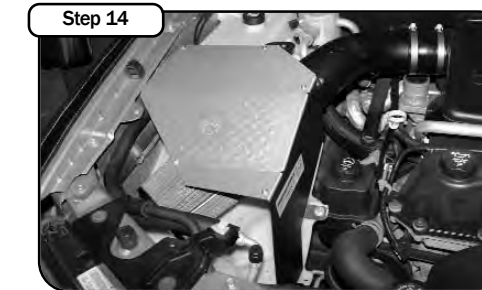
Step 14 Position the housing cover and secure in position using 4 button head screws. Your installation is now complete. Make sure you tighten all clamps and check all electrical connections. Re-check periodically.
