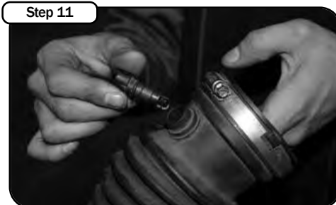
Step 11 Remove the air temp. sensor from the OEM intake tube.
