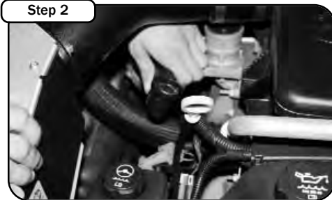
Step 2 Using wire cutters remove the factory metal clamp from the air injection hose.
