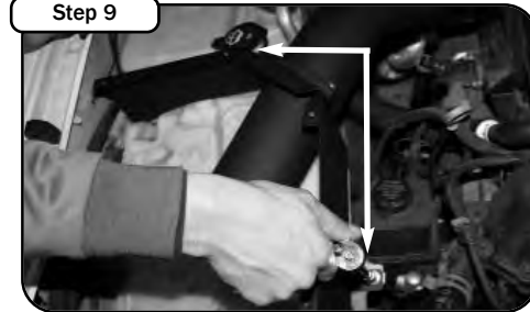
Step 9 Fit the aFe housing over the intake tube. Using 2 screws, washers and lock washers secure the housing in the engine compartment.
