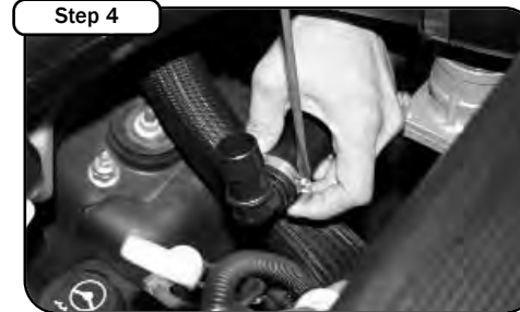
Step 4 Using the #12 clamp and supplied vent elbow, secure onto the air injection hose.
