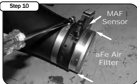
Step 10 After you aligned and inserted the MAF sensor, tighten the clamp. Insert and secure the aFe air filter onto the MAF sensor.
