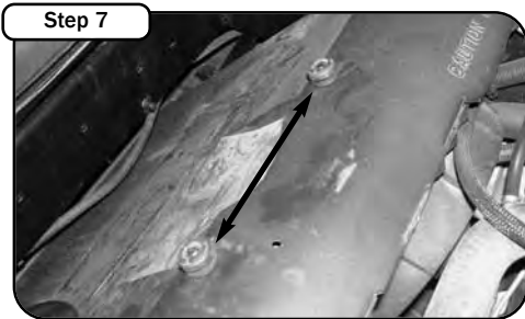
Step 7 Place the two rubber grommets on the two pins located on the engine cover.
