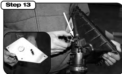
Step 13 Using the pliers to remove the two hose clamps on the OEM upper housing. Clip them onto the aFe housing cover.
