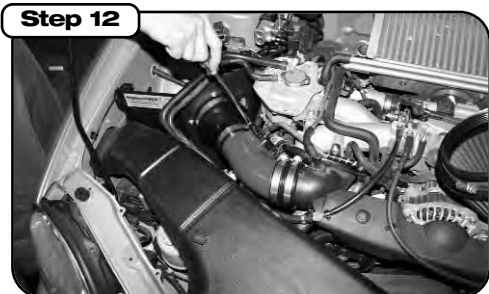
Step 12 Place the straight coupler & clamps on the aFe intake tube. Slide the coupler completely on the tube. Insert the tube into position, slide the coupler over and secure the clamps & housing. Plug in the MAF sensor.
