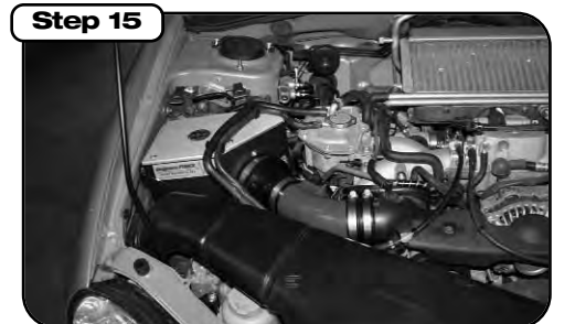
Step 15 Place enclosed CARB EO sticker on a clean/smooth surface on or near the intake system. EO identification label is required in passing the Smog Check inspection. Your installation is now complete. Make sure to tighten all clamps and check all electrical connections. Re-check periodically.
