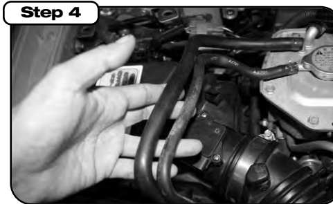
Step 4 Pull-up the two tubes located on the upper air box.
