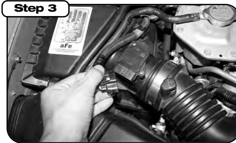
Step 3 Unplug the MAF sensor.
