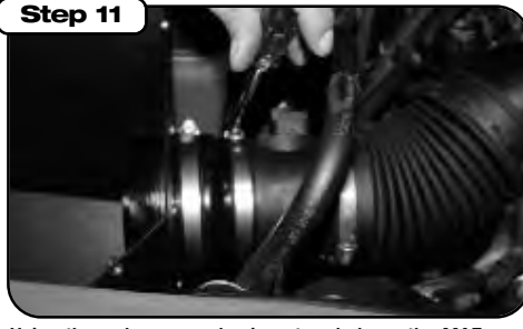
Step 11 Using the reducer coupler, insert and clamp the MAF sensor onto the aFe housing.
