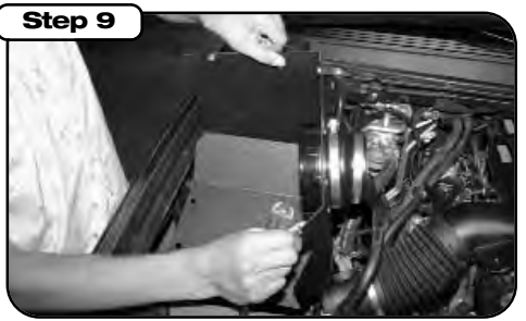
Step 9 With the filter adaptor and reducer coupler installed, lower the aFe intake housing into the engine compartment.
