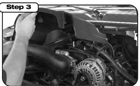
Step 3 Remove engine cover, lift up and pull out.
