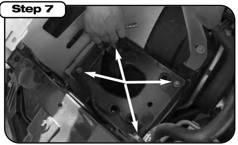
Step 7 Remove the 4 bolts that fasten the airbox mounting plate. Remove the plate and save the bolts for later use.
