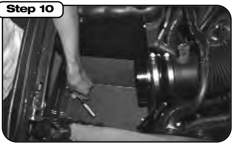
Step 10 Using the 4 bolts from the stock mounting plate fasten the aFe intake housing to the chassis.
