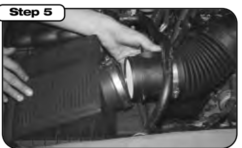
Step 5 Remove the MAF sensor from the housing.
