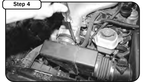
Loosen the two hose clamps from the intake plenum. Remove plenum from vehicle.
