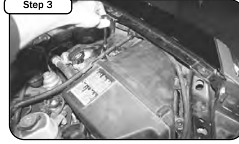
Remove the three screws that secure the air box to the vehicle.
