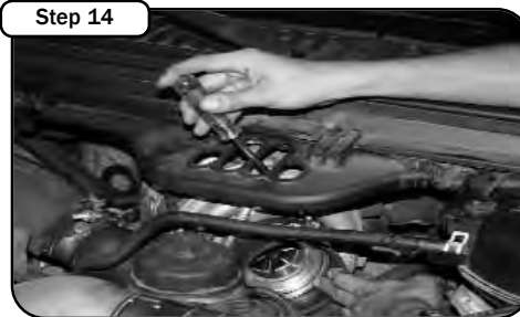
Step 14 Install grey high temp silicon coupling onto turbo. Tighten clamp at turbo.
