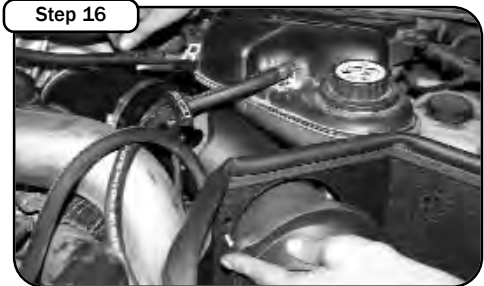
Step 16 Install tube and mount to housing using hardware provided. Tighten hump coupler where the two tubes meet.
