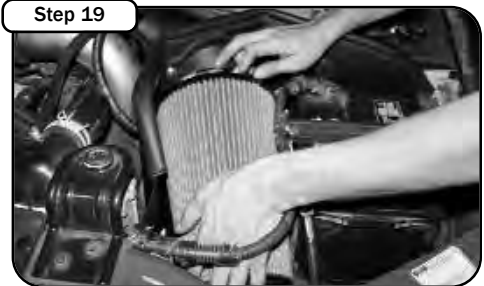
Step 19 Install filter onto tube. Tighten clamp.
