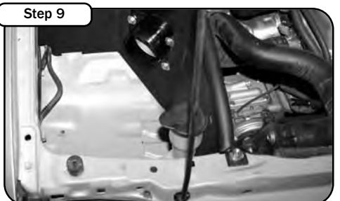
Lower housing into place. Secure the housing with provided screws (M8 and M6) using 10mm and 12mm socket. Re use 10mm bolt from step 6 , to secure front of housing onto radiator support.
