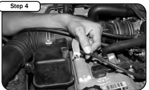
Disconnect and remove both vacuum lines from factory tube and loosen both clamps with 10mm socket or wrench.
