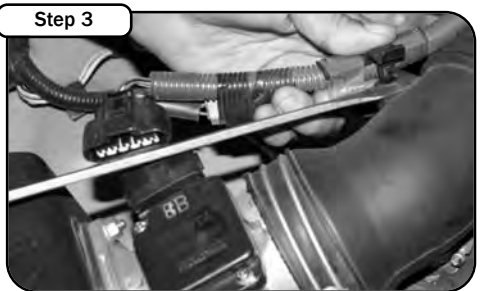
Disconnect negative battery terminal. Disconnect MAF sensor harness and remove wire from tube.
