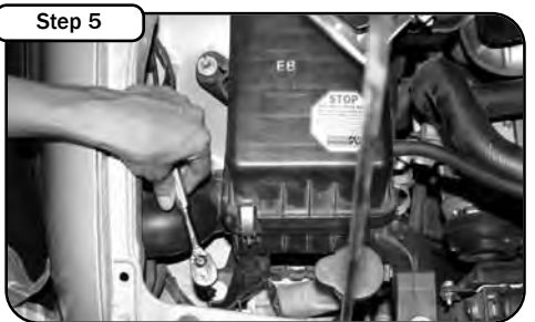
With 12mm socket loosen the 3 bolts holding the factory air box.
