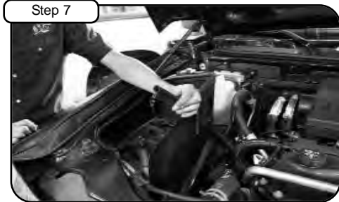
Step 7 Install 3/4 bulb trim seal on to top of aFe housing.
