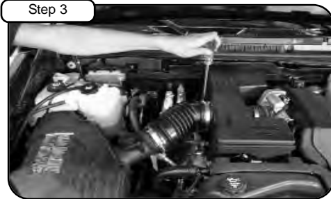
Step 3 Disconnect MAF sensor. With 5/16 nut driver loosen factory intake tube.
