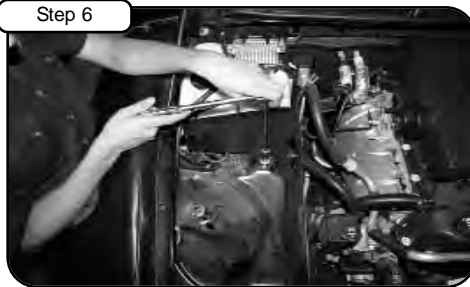
Step 6 Place new housing into vehicle. With the supplied screws, tighten using 10mm and 13mm socket.
