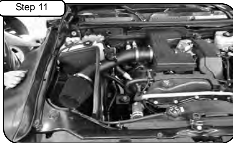
Step 11 Install 4" aFe high flow air filter to tube. Tighten all clamps with 5/16 nut driver. Re-connect MAF sensor. Your installation is now complete. Check and re tighten periodically.
