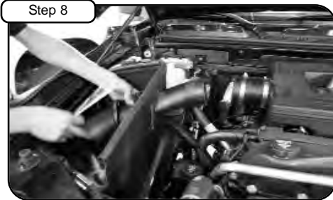
Step 8 Install hump coupler onto factory plenum box with clamps. Place tube through housing on to the coupler.
