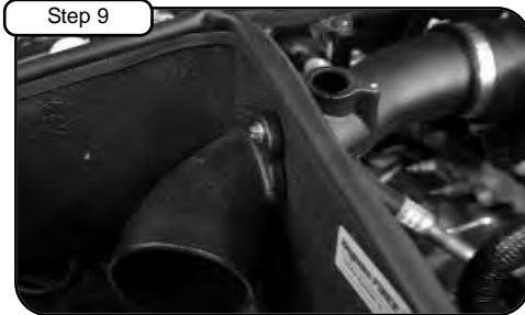
Step 9 With supplied screws, mount new tube onto housing using 10mm socket or wrench.
