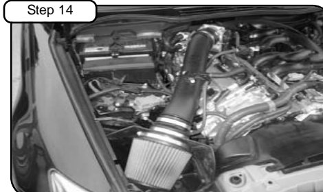
Step 14 Install new pre-oiled air filter onto adapter in housing. Tighten using 5/16 or slotted screwdriver. Re-connect MAF sensor harness. Carefully Re-install OE engine covers from steps 3 and 4.
