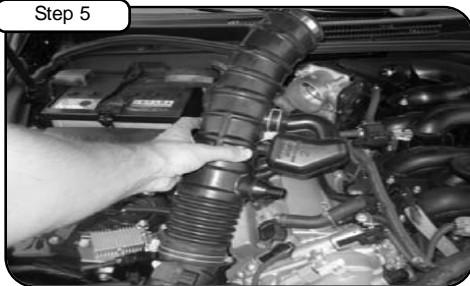
Step 5 Disconnect MAF sensor, w/ 10MM socket or wrench, loosen both clamps on factory intake tube. Carefully disconnect Crank case breather from tube and pull out the OE factory tube.
