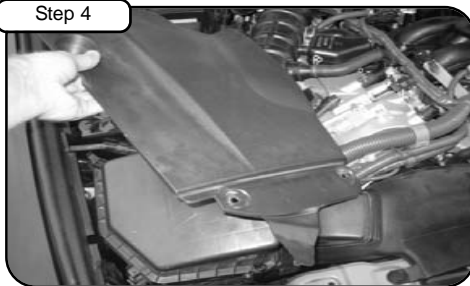
Step 4 Remove engine cover by pulling away from engine, remove the 1 remaining push clip from intake cover.
