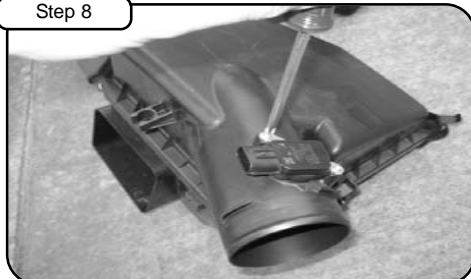
Step 8 With phillips screwdriver un-screw the 2 bolts holding MAF sensor, CAREFULLY pull out sensor.
