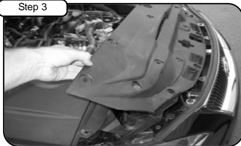
Step 3 Carefully Remove 12 plastic push clips of the front engine cover. Set aside to re-install later when finished
