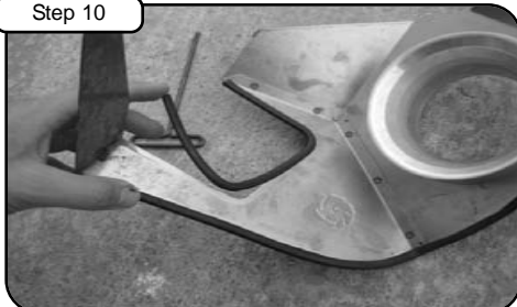
Step 10 Install 5 1/2" adapter to housing using 3 button head screws with 5/32 allen wrench. Apply trim rubber edge seal to bottom and 7/16 bulb seal to top of housing.
