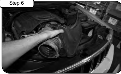
Carefully remove upper half of OE airbox and plenum intake box.
