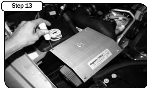
Install housing cover using button head screws provided. Tighten using 5/32" allen key.
