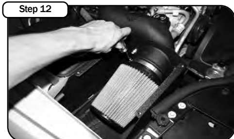
Install filter onto intake tube and tighten using 5/16" nut driver.
