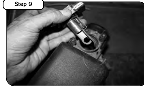
With phillips screwdriver, carefully remove the mass air sensor from OE airbox.
