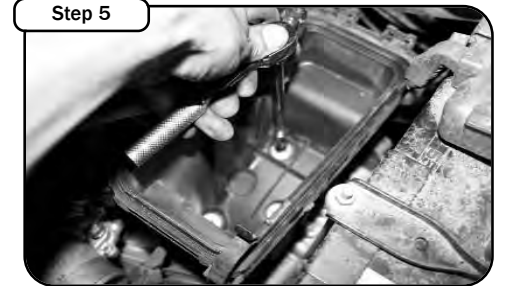
Loosen the 3 10mm bolts with socket and extension holding the lower part of air box. Also, remove the 10mm bolt holding the OE snorkel next to battery.
