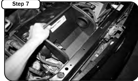
First, loosen 10mm bolt located under radiator support on left hand side of vehicle and remove. Place trim seal onto housing and install into front of vehicle. Replace bolt into vehicle with housing and tighten.
