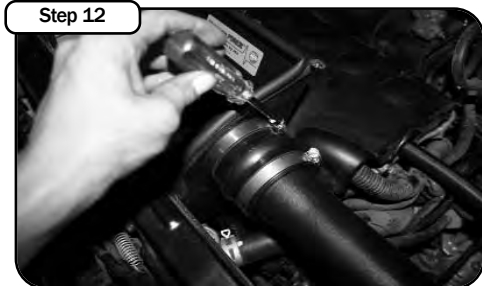
Tighten using 5/16" nut driver on both ends at throttle body and housing side. Re-connect MAF sensor harness.
