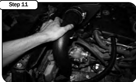
With couplers and clamps provided place onto both ends of tube and place into vehicle.
