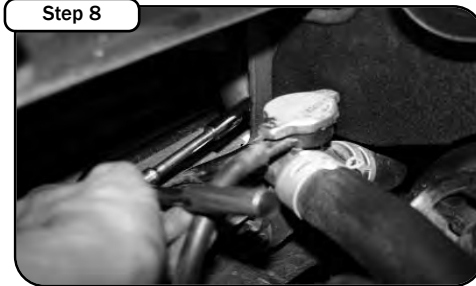
With M6 screw and washer provided, tighten housing through grill support.
