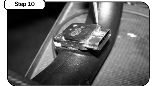
Place mass air sensor into new tube with gasket and nylon spacers provided between tube and sensor. Tighten using M4 screws provided.
