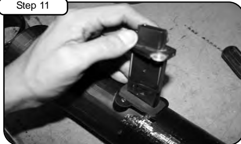
Re-insert MAF sensor into new intake tube. With gasket and nylon spacers provided, place in between tube and sensor. Tighten with screws provided.
