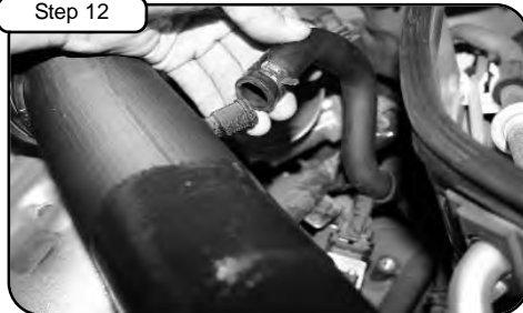
Place aFe tube inside vehicle. Re-insert crankcase line onto new tube.
